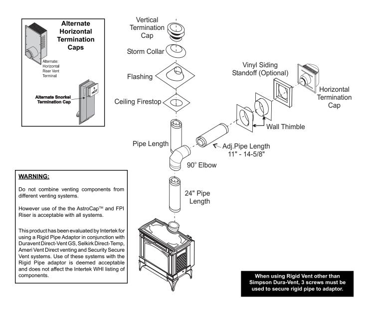
The FPI AstroCap<sup>™</sup> and FPI Riser Vent terminal are certified for installations using FPI venting systems as well as Simpson Dura-Vent<sup>®</sup> Direct Vent GS, American Metal Products Ameri Vent Direct Vent, Security Secure Vent<sup>®</sup>, Selkirk Direct-Temp. AstroCap<sup>™</sup> is a proprietary trademark of FPI Fireplace Products International Ltd. Dura-Vent<sup>®</sup> and Direct Vent GS are registered and/or proprietary trademarks of Simpson Dura-Vent Co. Inc.
